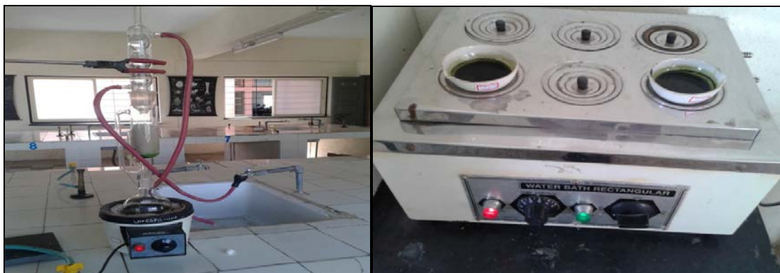
Figure 2: Soxhlet extraction apparatus and electronic water bath
